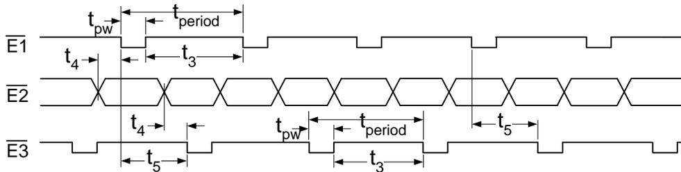
**Figure 2. Timing Diagram for  $\overline{E1}$ ,  $\overline{E2}$ , and  $\overline{E3}$**
