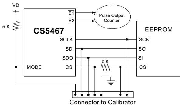
**Figure 13. Typical Interface of E<sup>2</sup>PROM to CS5467**
