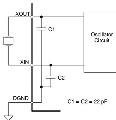
Figure 7. Oscillator Connections
